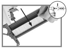
Figure 3. Loading nails into magazine.
